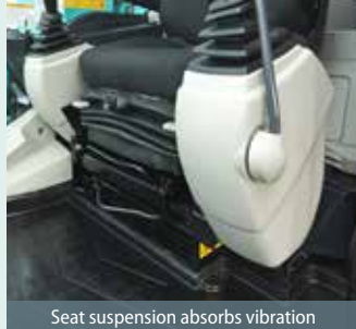
Seat suspension absorbs vibration
