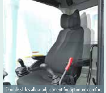
Double slides allow adjustment for optimum comfort
