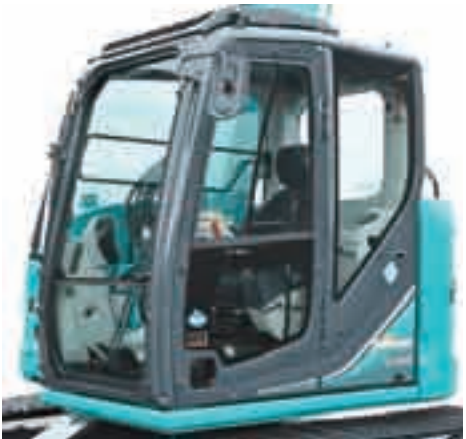
*Photo is the optional specs with FOPS guard.
